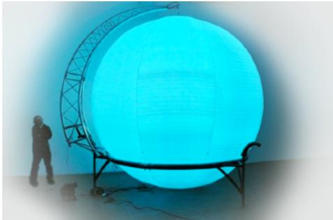
A 4-metre diameter inflated sphere sits on a 3m diameter metal frame with three adjustable height legs.
